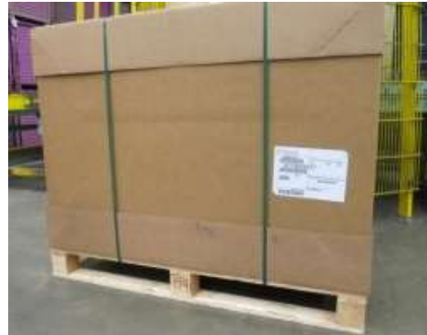
Attached to cardboard boxes, strapping does not obscure goods label
