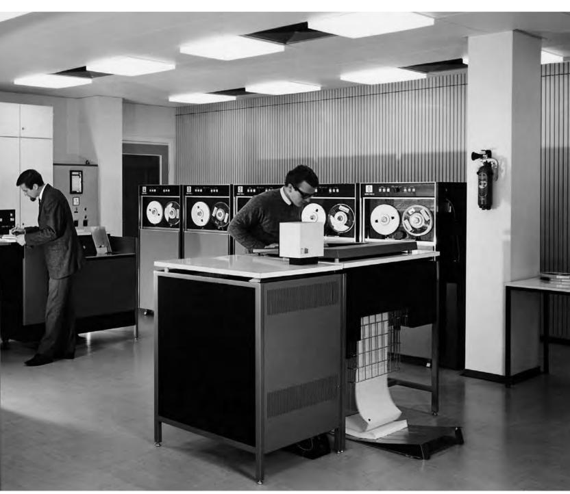
**A NEW AGE /** In 1967, computers were deployed for the very first time at Mann + Hummel for electronic data processing. The bulky technology was housed in a rented premises of the textile plant, the "high-speed printer" produced 27,000 lines per hour.
