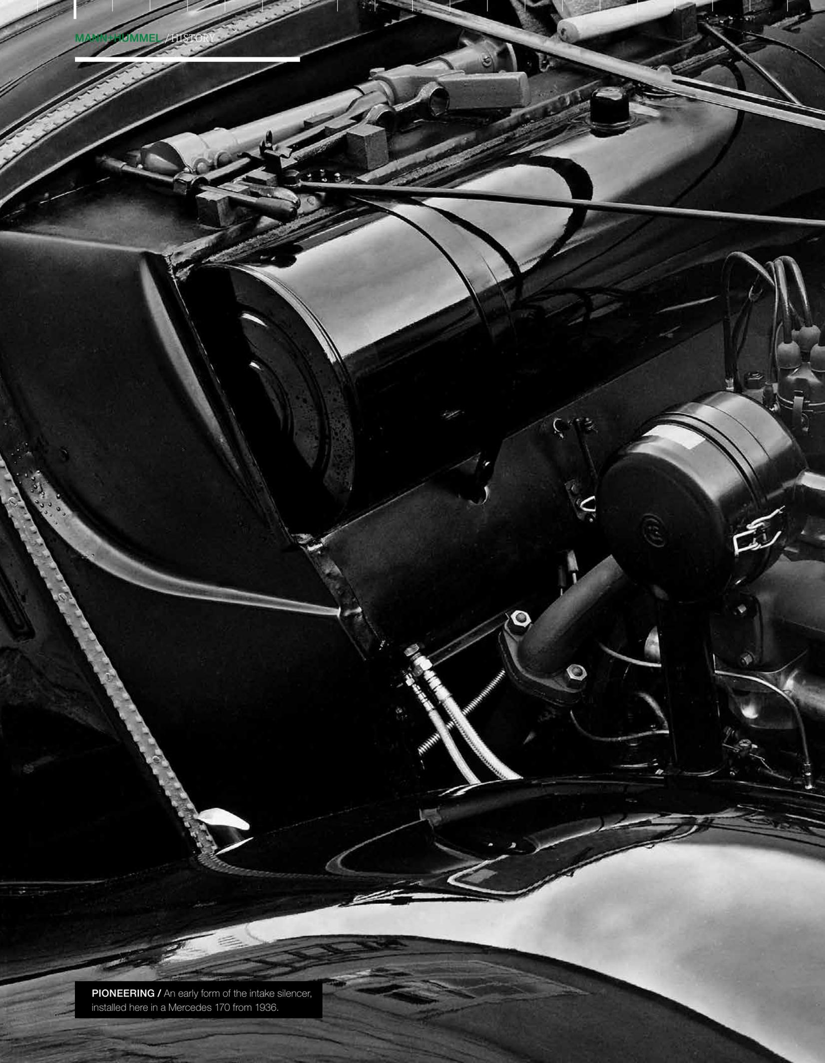
**PIONEERING** / An early form of the intake silencer, installed here in a Mercedes 170 from 1936.
