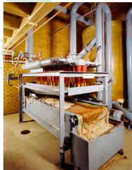
**HYDROCYCLONE SYSTEM** / Section of a MANN hydrocyclone system for the cleaning and recooling of the cooling emulsions of wire drawing machines.
