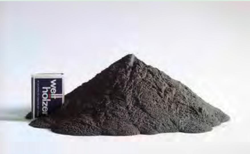
**A PICTURE IS WORTH A THOUSAND WORDS /** This advertising photo from 1993 shows how much air filter dust a bus accumulates over 10,000 kilometers.
