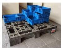
The KLT Lego Bottom standard boxes allow the stacking in the way the bottom fitting avoid displacements during the transportation and unloading.
