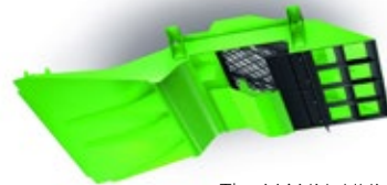
The MANN+HUMMEL fine dust particle filter mounted on the underbody of the vehicle
