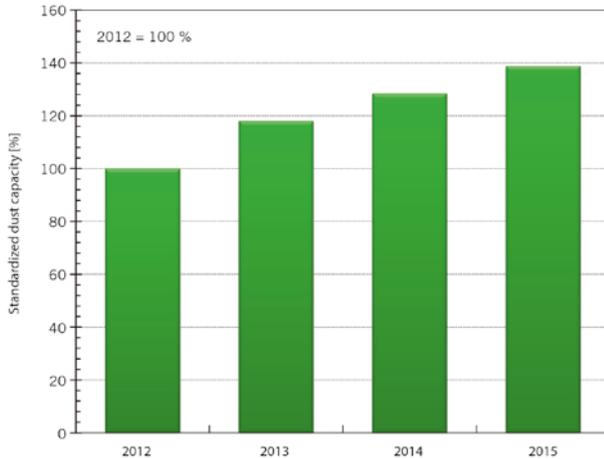
FIGURE 3: Development of volume-specific dust capacity of fleece media (© MANN+HUMMEL)
