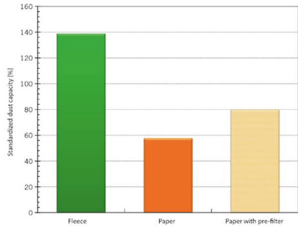
FIGURE 4: Comparison of dust capacity of fleece and paper air filters (© MANN+HUMMEL)
