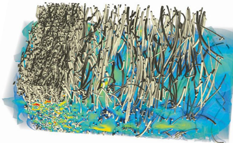
FIGURE 5: CFD simulation of the flow field through a fleece medium for material optimization, based on X-ray tomographs (© MANN+HUMMEL)
