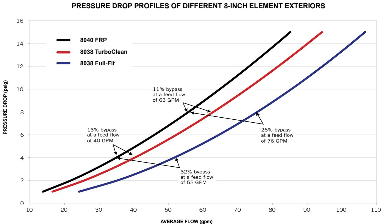
As shown in the chart above, TurboClean® elements allow less flow to bypass the element, resulting in higher cross-flow velocity at the membrane surface. TurboClean elements typically exhibit about 12% bypass flow—60% less than the 30% bypass flow from competitive full-fit elements.
